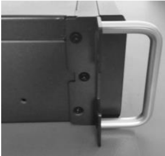
FIGURE 4 Attach the mounting bracket and handle
